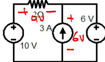
$$\begin{aligned}P &= VI \\&= 4 \times 2 \\&= 8 \text{ W}\end{aligned}$$
